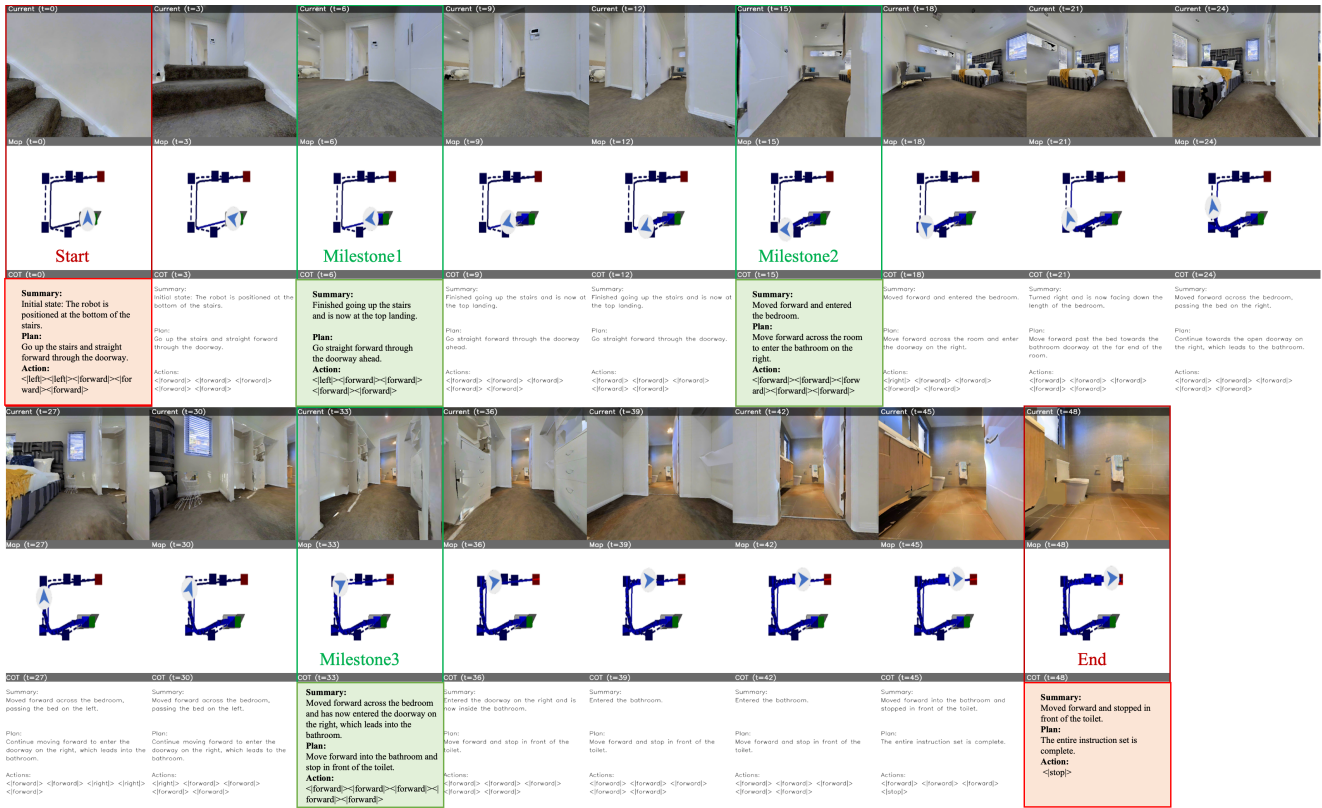
Figure 6. Hierarchical planning examples generated by NavForesee for the instruction "Go up the stairs and straight forward the doorway. Turn right, move forward, and enter the doorway on the right. Move forward into the bedroom and stop in front of the toilet". From top to bottom: frames with timestamps, global navigation map, and navigation planning outputs. NavForesee accurately identifies milestones along the route, summarizes completed sub-instructions, and generates the next sub-instruction in accordance with the instruction context.
