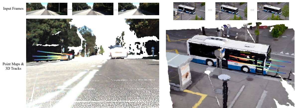
Figure F. Qualitative visualization of 3D point tracks, obtained by our method, over time steps.
