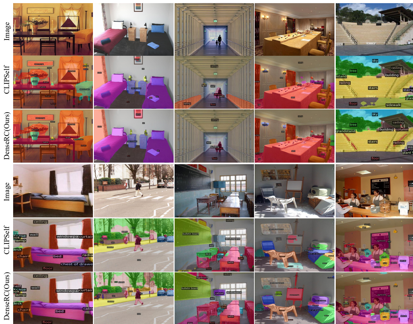
Figure 7. Visualization of open-vocabulary semantic segmentation results on ADE20K (A-150).
