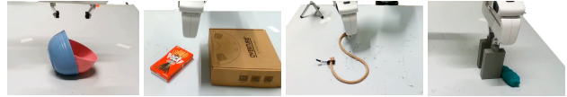
Figure 14. Failure cases. Example failure cases in bowl stacking, pivoting, shape rope and shape dough tasks.
