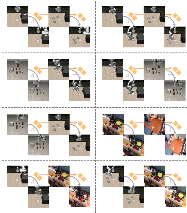
Figure 5. Transfer linear interpolation experiment with the StaMo encoder. The left and right panels illustrate different task scenarios, where reconstructions are obtained by \text{tokens}(3) + \text{tokens}(2) - \text{tokens}(1) , demonstrating the linear interpolation property of latent representations during transfer.
