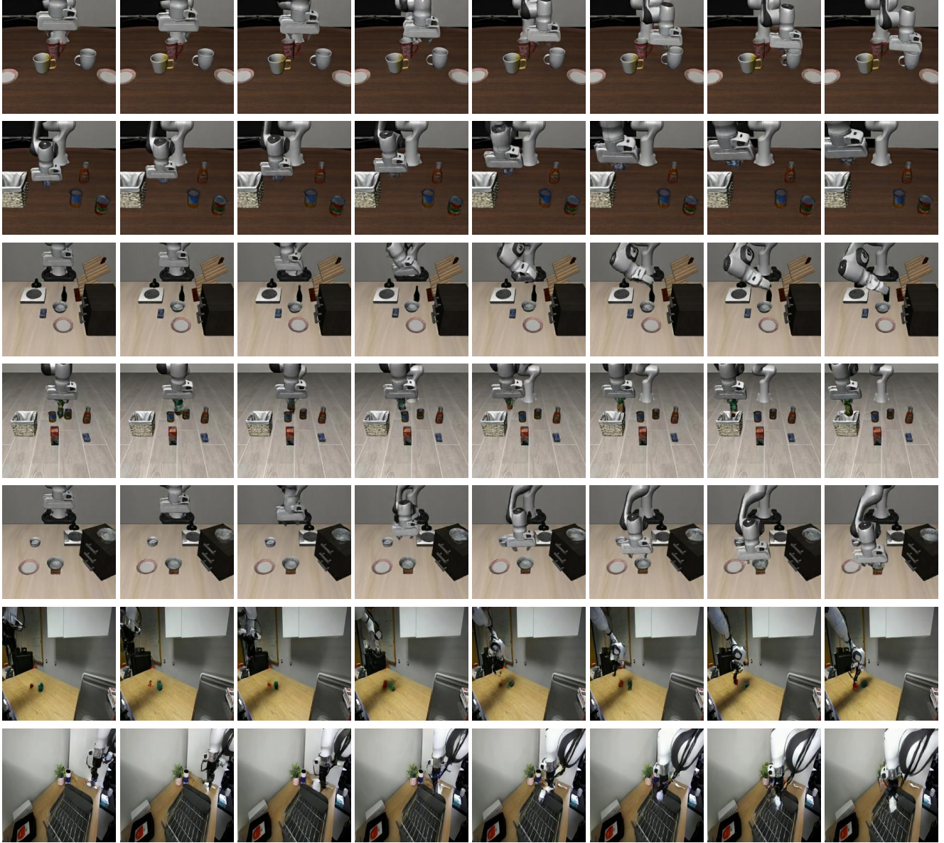
Figure 4. Visual reconstruction results from the same episode. The first and last frames are reconstructed from ground-truth images using the StaMo encoder, while the intermediate frames are generated by linearly interpolating between the latent state tokens of the two endpoints. The transitions show that both the robotic arm and the objects move in a continuous and smooth manner.
