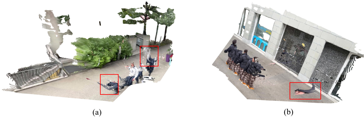
Figure 6. Common failure modes of directly reconstructing humans as raw geometry. (a) Dynamic body motion and complex clothing often lead to fragmented or noisy human surfaces. (b) Articulated limbs may be misclassified as background, causing them to merge into the static scene. These artifacts motivate our use of the SMPL model, which provides a structured human prior and avoids such degeneracies.
