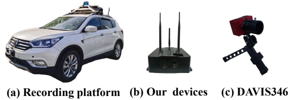
Figure 5. Data collection setup. (b) Our custom synchronized capture device is mounted on the (a) vehicle platform to record DrivTAP, and (c) a DAVIS346 camera is used to collect the InivTAP dataset.
