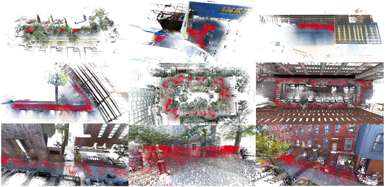
Figure II. Our 3D reconstruction from LIV-SLAM. The global colored point cloud is downsampled for visualization cleanness.
