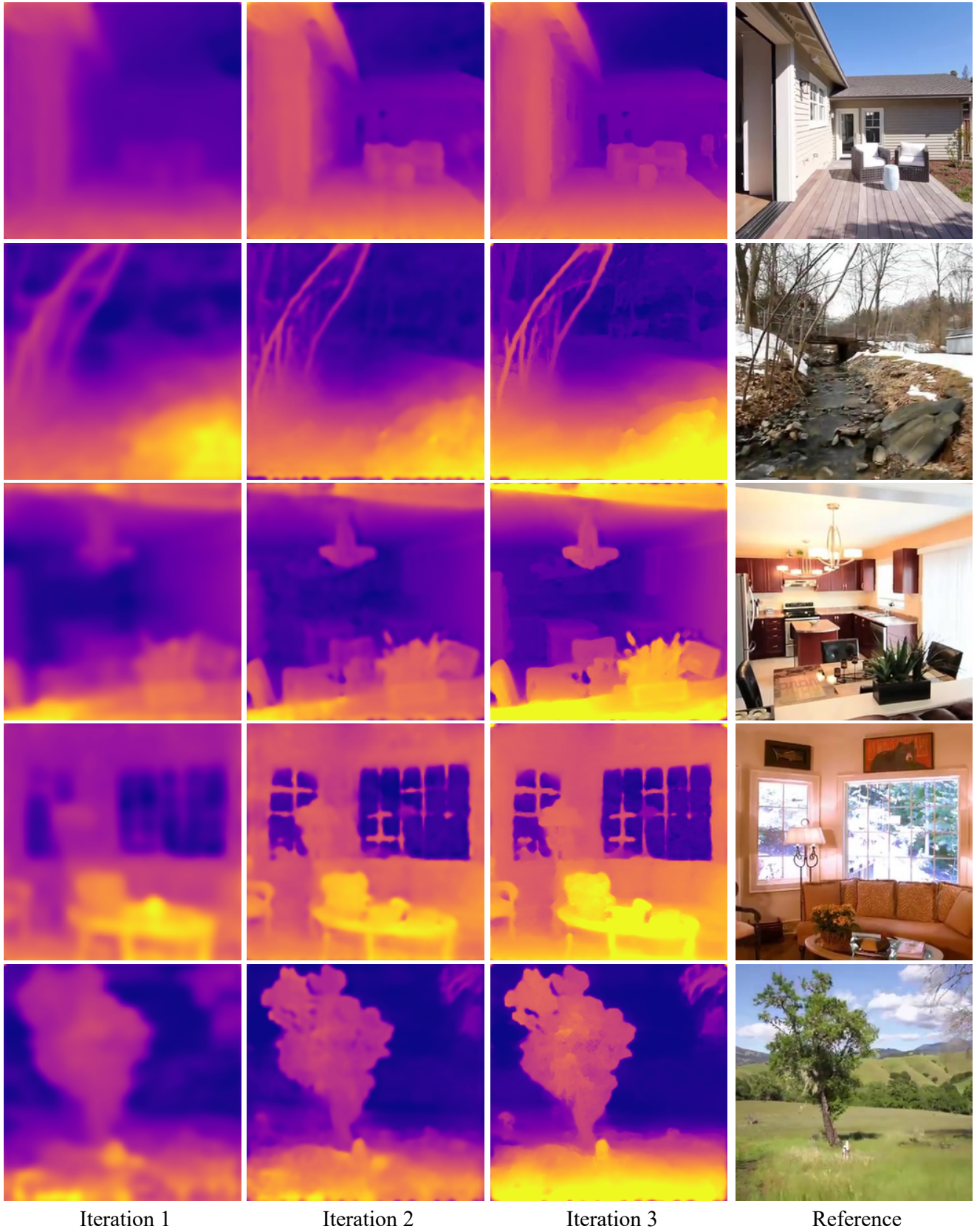
Figure 12. Visualization of intermediate depth prediction maps at different iterations in the IDESplat network.
