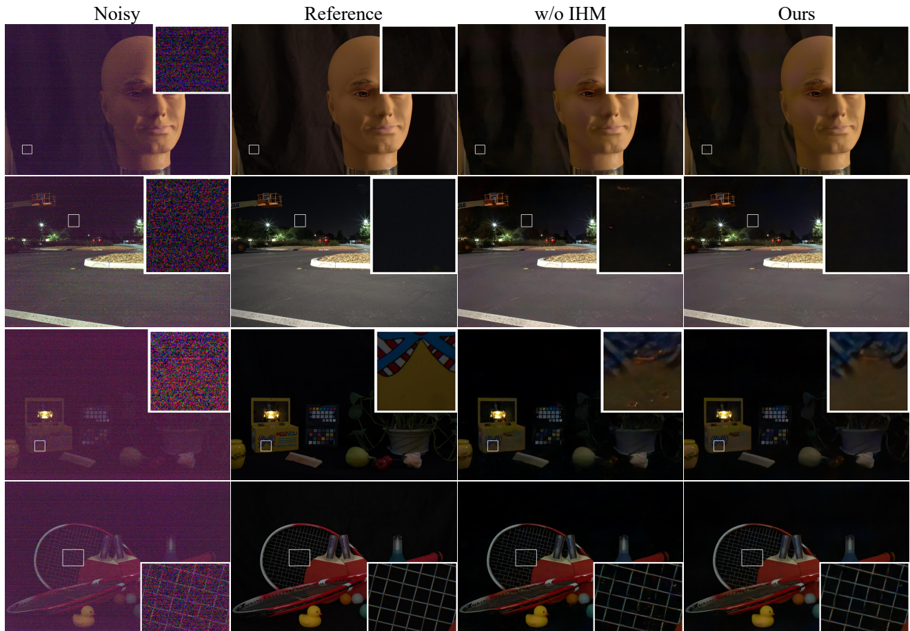
Figure 11. Ablation study on the iterative histogram matching (IHM). Without IHM, noticeable white spots appear in the denoised outputs due to saturated pixels in the noisy inputs. With our full method, this issue is effectively mitigated. The first two examples are from the SID test set while the third and fourth are from the ELD test set. Best viewed zoomed in.
