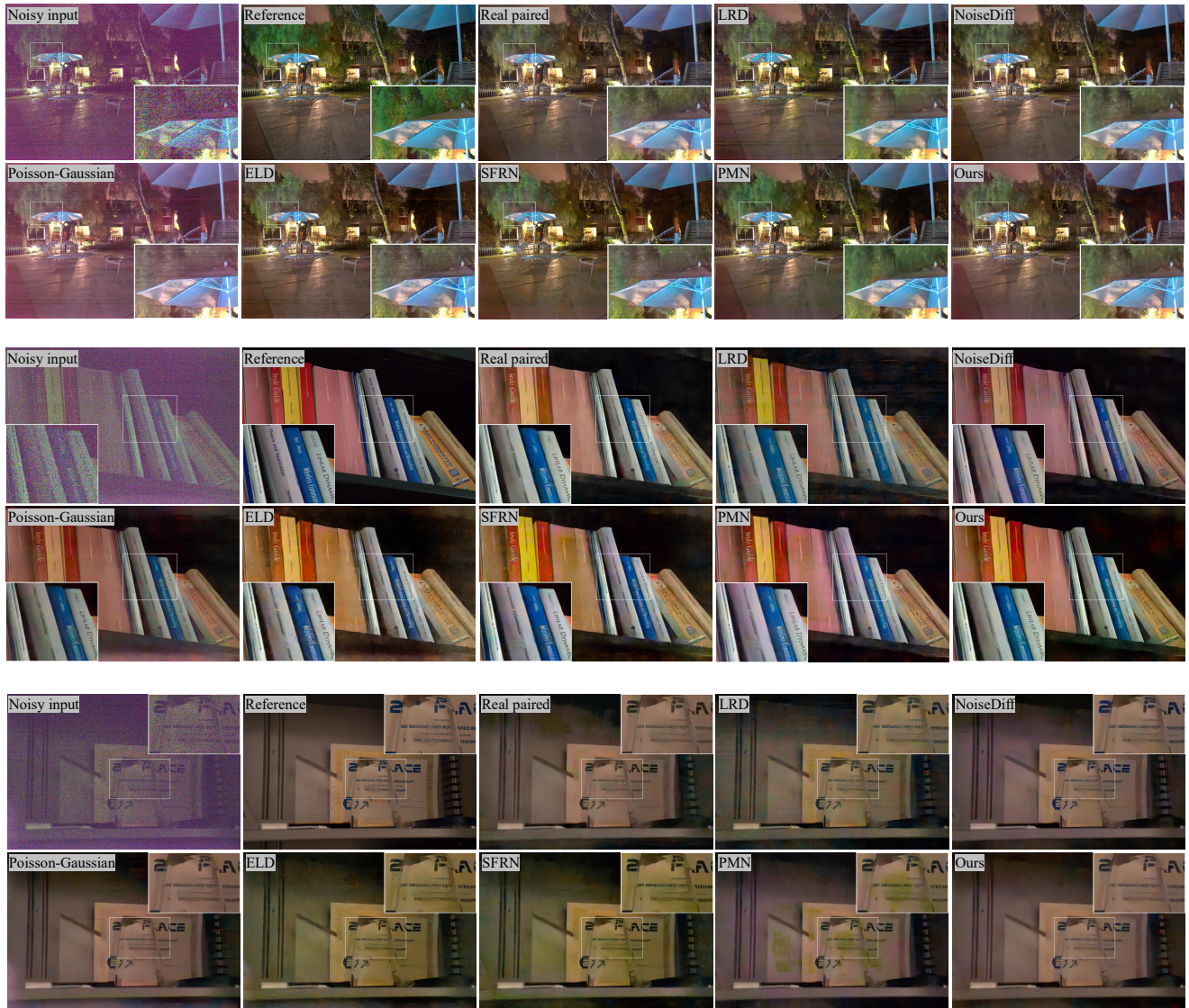
Figure 18. Result comparison of denoisers trained on data synthesized using different methods on the SID test set.
