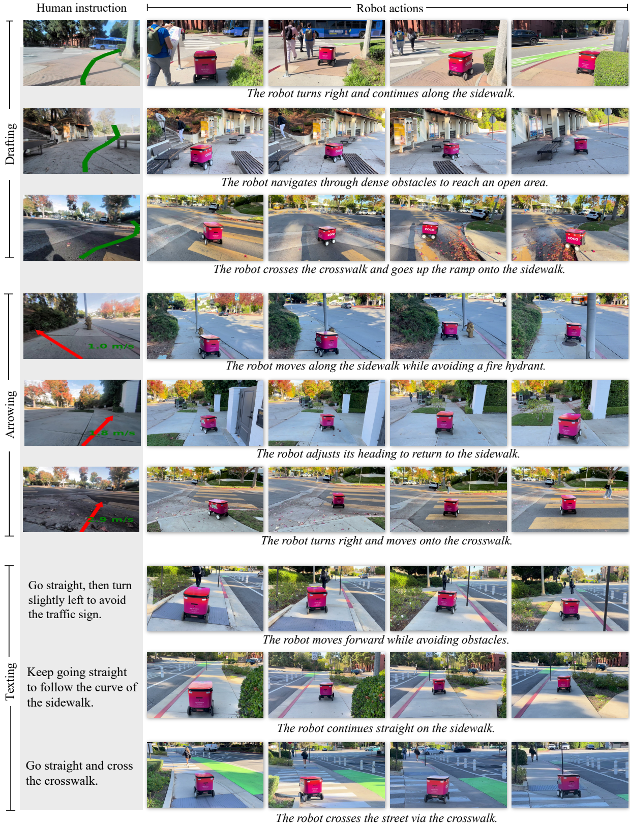
Figure 18. Qualitative results in the real world. The first three rows are guided by drafting, rows 4 to 6 by arrowing, and the last three rows by texting. The first column shows human instructions, while columns 2 to 5 show the actions executed by the robot.
