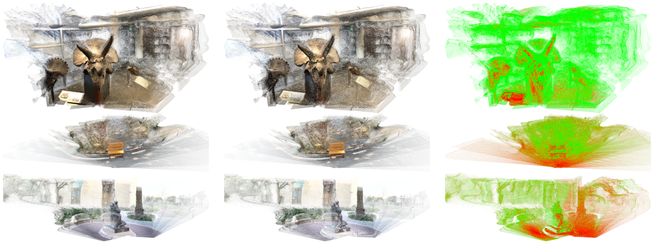
Figure 6. Comparison of point clouds on three datasets: LLFF, MVImgNet, and Tanks and Temples (rows). Each row shows results from InstantSplat (left), our BA-GS method (middle), and their overlay: InstantSplat (Red), BA-GS (Green).
