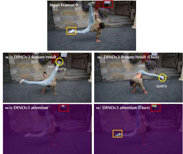
Figure 8. Visualization of attention maps. We visualize the responses of the first input frame to a selected patch (yellow circle) in an interpolated frame. Previous attention modules extract patches only based on pixel similarities and distance, thus only response to the white backboard in the red boxes. In contrast, our attention module can extract patches based on motion information by DINOv3 patch similarities, enabling the model to generate correct motions rather than simple pixel-wise approximation.
