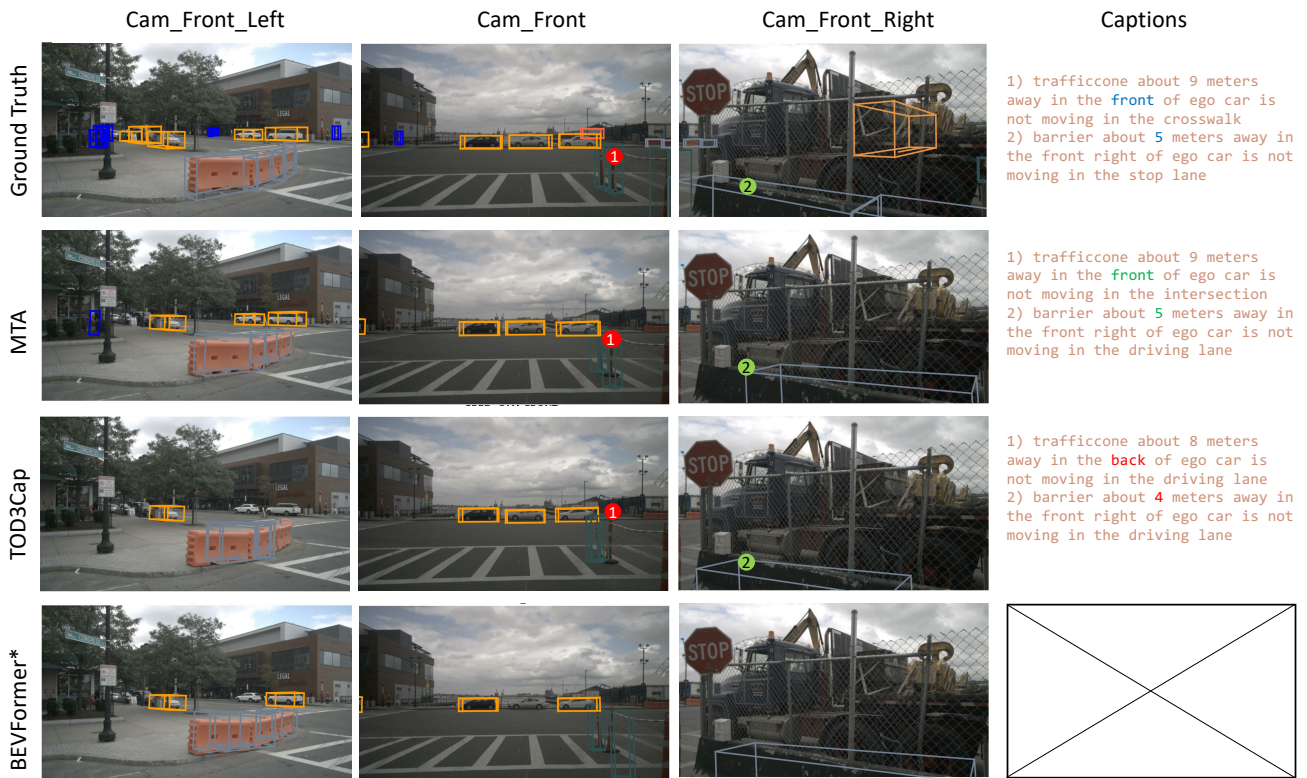
Figure 3. Qualitative results comparing the proposed MTA with baseline methods on nuScenes and TOD3Cap datasets. Visualization results show that MTA shows improved alignment with ground-truth detections over the counterpart methods. Captioning results show that the proposed MTA generates captions that are more accurate in terms of description and spatial orientation of objects over the TOD3Cap. Unlike MTA, TOD3Cap perceives object 1 (a trafficcone) to be positioned in the back of the car instead of front in the caption, illustrating a heightened risk of hallucination. *We note that BEVFormer is only suited for perception tasks, thus caption is not provided.
