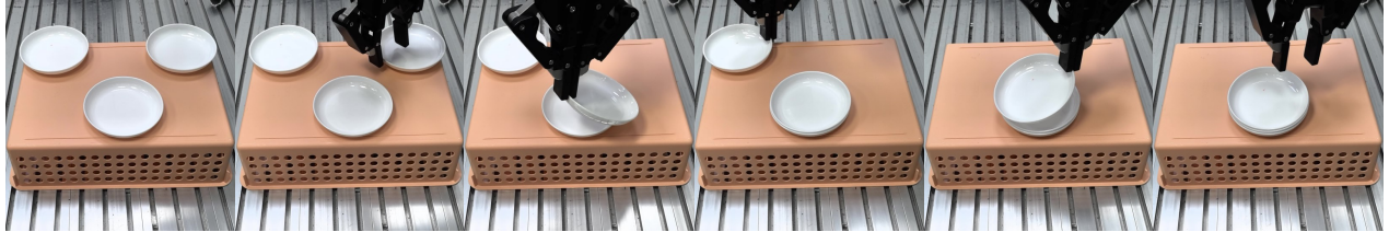
Figure 8. VITA executes the “Stack Plates” task. Following the instruction (e.g., “Stack the plates one by one”), VITA controls the gripper to stack them sequentially. This process demonstrates VITA’s planning and execution capabilities in multi-step manipulation and physical interaction.
