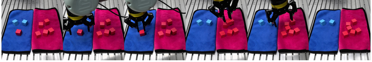
Figure 7. VITA executes the “Color Matching” task. Following the instruction (e.g., “Place red and blue blocks on towels of matching colors”), VITA controls the gripper to place the red block on the red towel and the blue block on the blue towel, successfully completing the classification.
