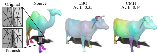
Figure 16. The tool we use to tetrahedralize surface matching datasets [43] is robust, but occasionally introduces topological noise, closing unwanted handles that alter the mapping task (closeup). The LBO eigenbasis is not robust against such defects. Conversely, the CMH basis is robust and greatly improves the mapping quality. Both the camel and the cow are from the SHREC’20 dataset.
