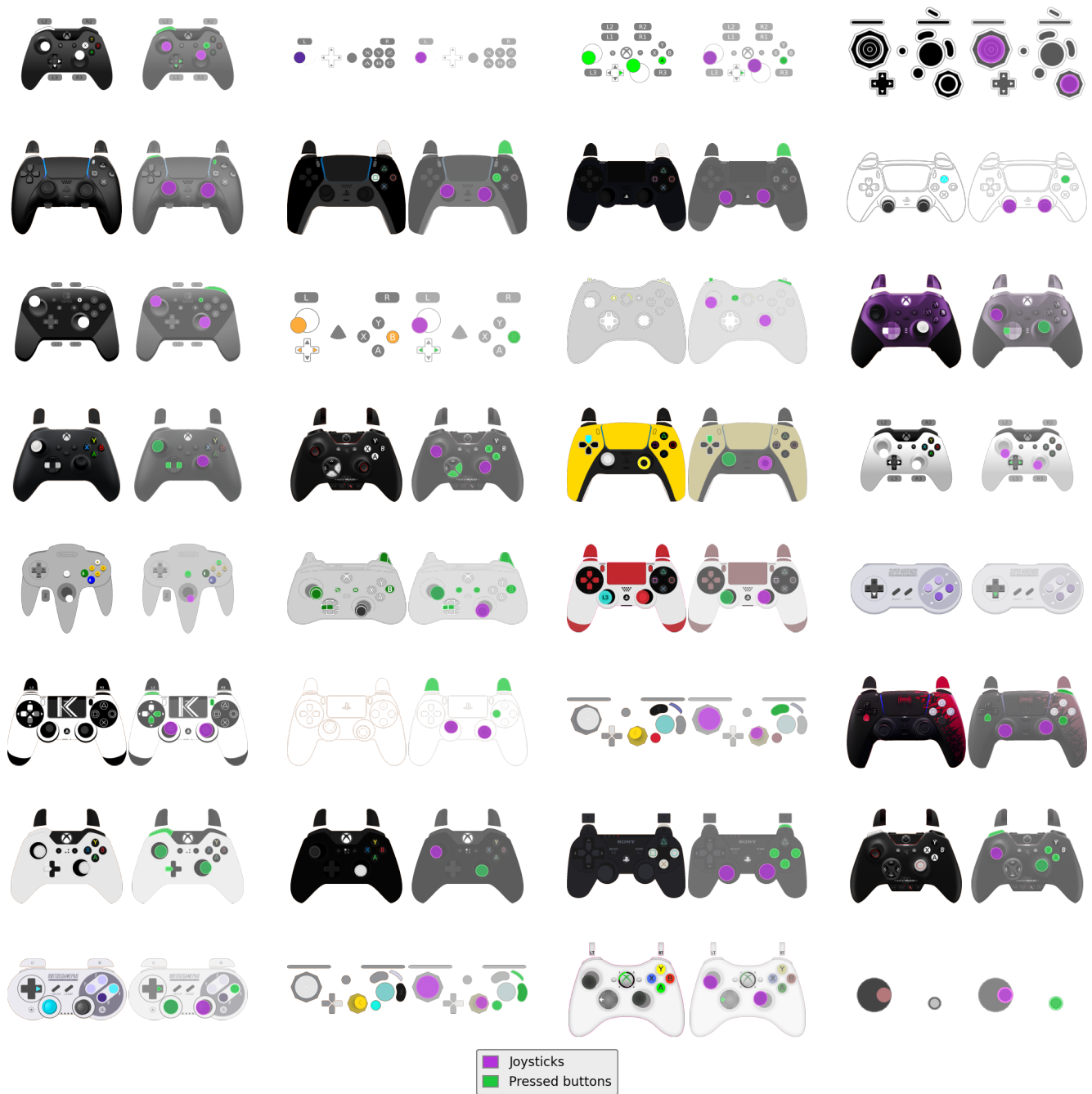
Figure 8. Synthetic controller overlays. We programmatically generate gamepad overlay images using existing controller overlay software, producing paired RGB frames, joystick segmentation masks, and ground-truth button states. The figure illustrates the diversity of controller overlay representations across software and skins. For each pair, the left image shows the raw overlay, while the right image highlights joystick segmentation masks (purple) and pressed buttons (green). These synthetic data are used to train our action labelling model.
