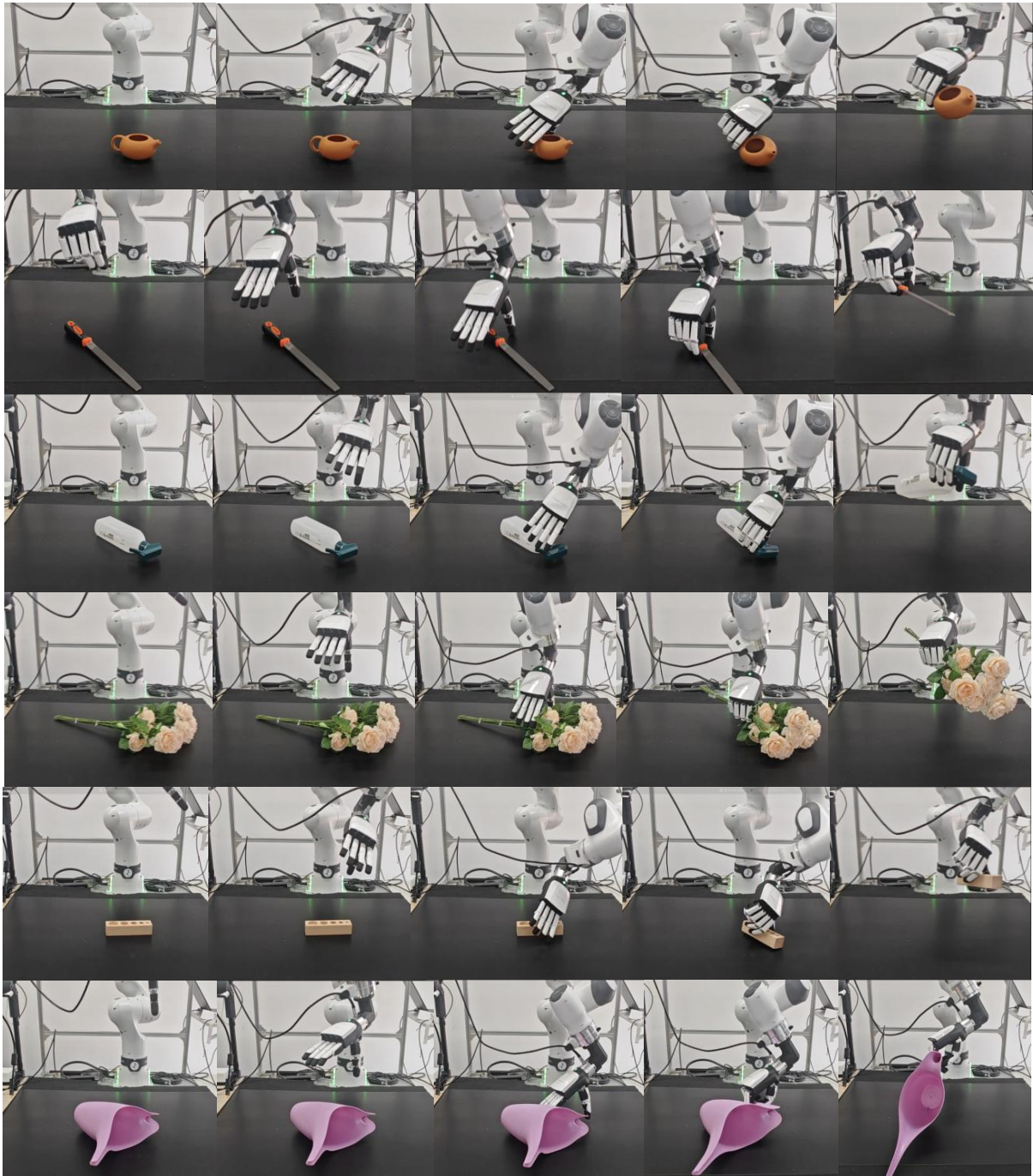
Figure 15. Real-world video recordings of the vision-based policy performing functional grasps on a variety of objects.
