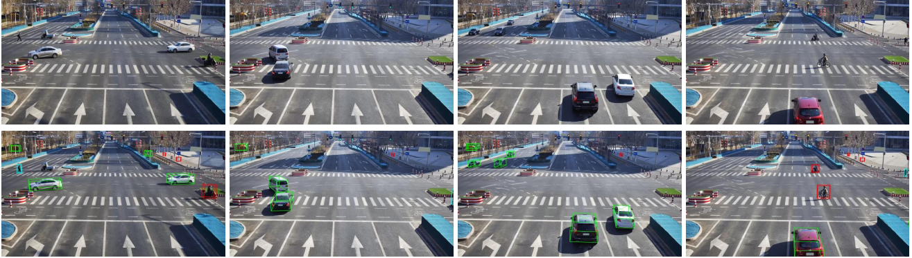
Figure 2. Training samples from DAIR-V2X-I selected during LH3D Stage 1 through depth-confident sample selection. The top row displays the original images, and the bottom row shows the corresponding 3D bounding box annotations. The samples selected during Stage 1 are characterized by high visual clarity and minimal ambiguity. The selection strategy prioritizes scenes where vehicles, pedestrians, and cyclists appear without occlusion and are positioned at moderate distances. Furthermore, these samples exhibit low scene complexity, avoiding overcrowded traffic environments.
