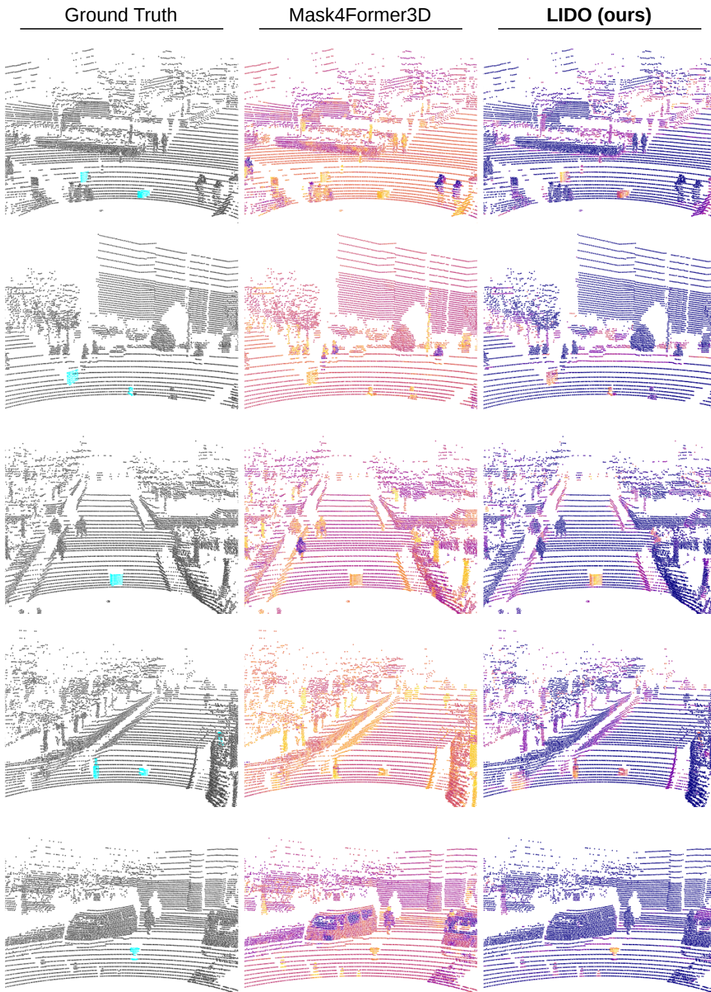
Figure 8. Qualitative comparison of 3D LiDAR anomaly segmentation results on SemanticPOSS-OoD Multi split.
