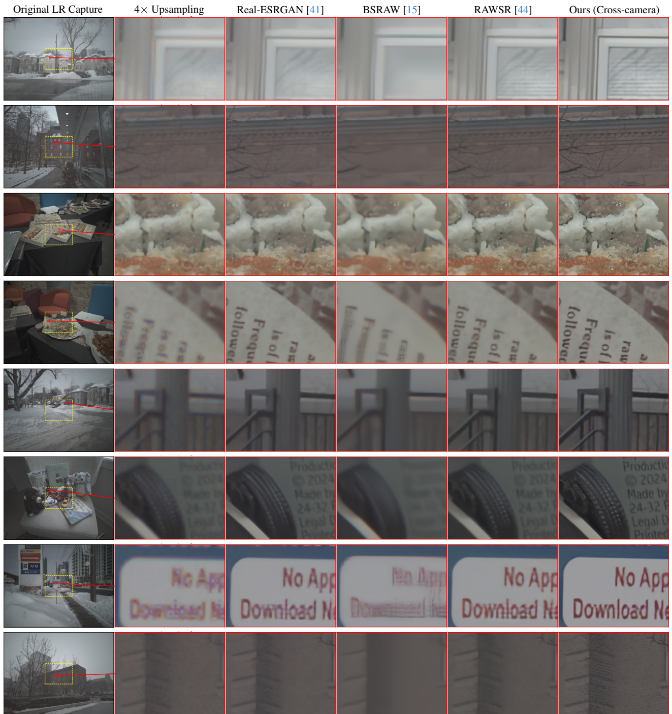
Figure S6. Additional qualitative results for 4× SR on Pixel 6 Main from the experiments in Sec. 4.5 of the main paper. Note that Pixel 6 Main degradations are not explicitly included in the training data of any of the models. Model outputs are white-balanced and gamma-corrected for better visualization.
