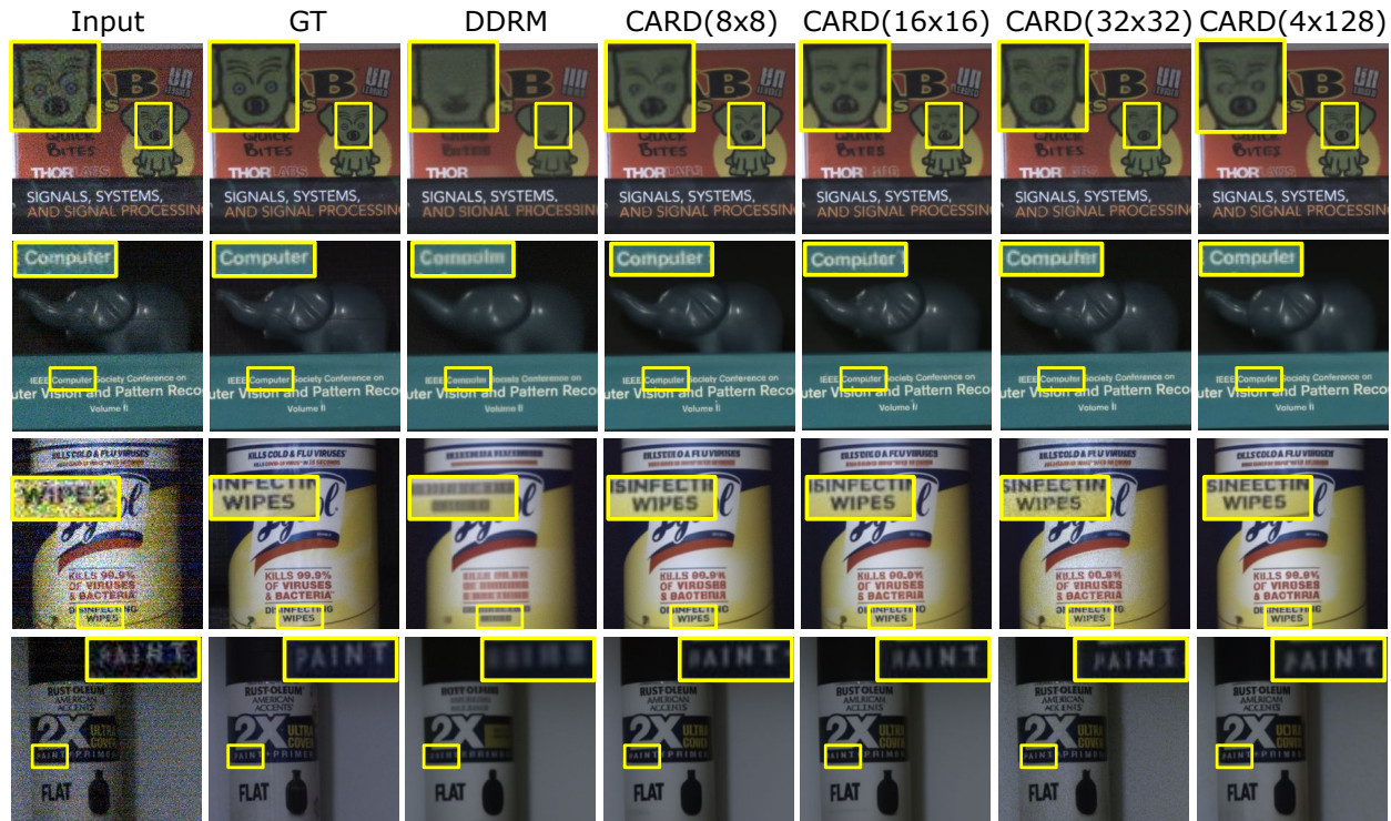
Figure 4. Effect of patch size on CARD denoising quality. Top two rows show low-noise images where smaller patches ( 8 \times 8 , 16 \times 16 ) produce slightly clearer outputs. Bottom two rows show high-noise images where larger and anisotropic patches ( 32 \times 32 , 4 \times 128 ) yield improved visual quality by better capturing spatial noise correlations.
