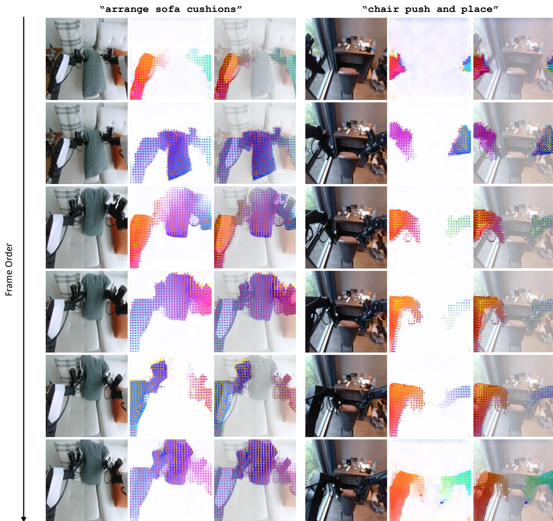
Figure 2. Galaxea-Open-World-Dataset pixel motion prediction examples. The first column shows the one test image sequence given the task of “arrange sofa cushions”. The second column shows the test image sequence given the task of “chair push and place”. Each group shows the original head-camera observation and the visualizations of corresponding pixel motions predicted by Motion Director.
