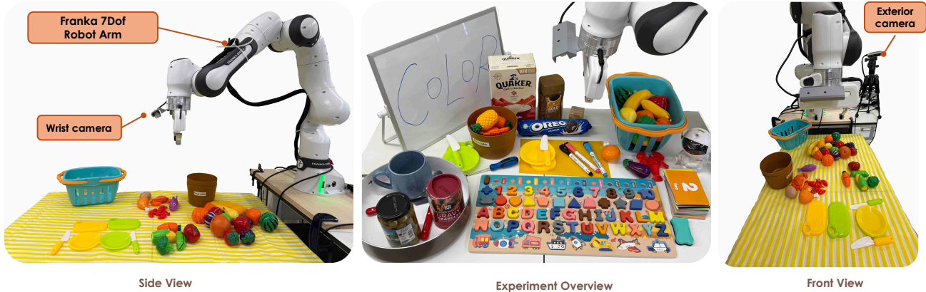
Figure 11. Real-World Robot Platform. Franka Research 3 manipulation system with dual Intel RealSense D435 cameras. Our experiments involve diverse everyday objects (vegetables, fruits, utensils, blocks) in realistic tabletop scenarios for long-horizon compositional and reasoning-intensive manipulation tasks.
