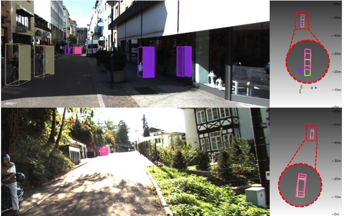
Figure 2. Visualization of candidate sets produced by RARE on the KITTI validation set. Each row displays the RGB image with projected 3D boxes (left) and the corresponding Bird's-Eye View (BEV) plot (right). For each RoI, RARE generates a compact set of candidates: for nearby objects, the hypotheses tightly align with the ground truth , whereas for distant objects, they exhibit variance along the depth axis in BEV, effectively capturing the inherent depth ambiguity. Legend: (Car, Cyclist, and Pedestrian).
