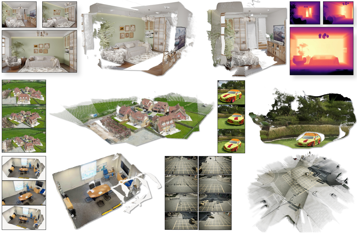
Figure 9. Feed-Forward 3D Point Map by OmniVGGT with In-The-Wild Inputs.
