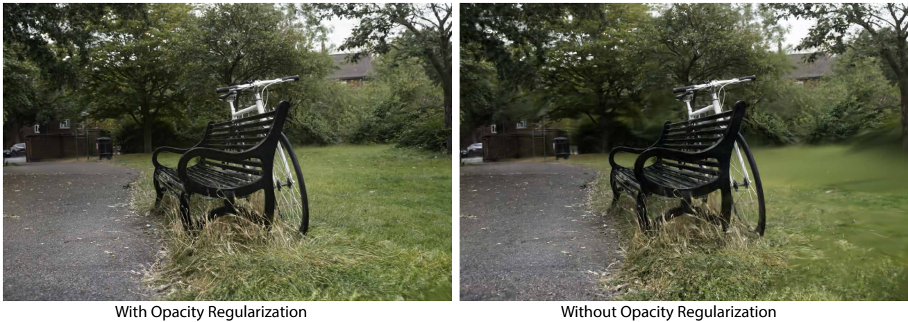
Figure S4. The results of our method with the opacity regularization (left) and without it (right). Opacity regularization prevents large high-opacity Gaussians from dominating regions such as distant grass, and enables preserves fine detail.
