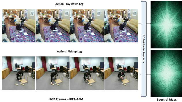
Figure 6. IKEA-ASM symmetric actions. 3D FFT spectra (right) distinguish lay down leg from pick up leg through subtle motion-direction cues that are hard to see in RGB space.
