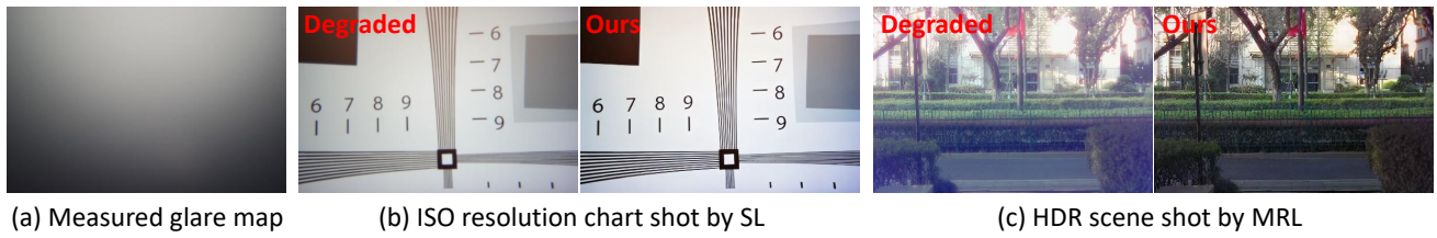
Figure 5. (a) Physically measured glare map ( I_c \approx 0 ). (b) High-frequency detail recovery on an ISO resolution chart (SL). (c) Robust veiling glare removal in a high-contrast HDR environment (MRL).
