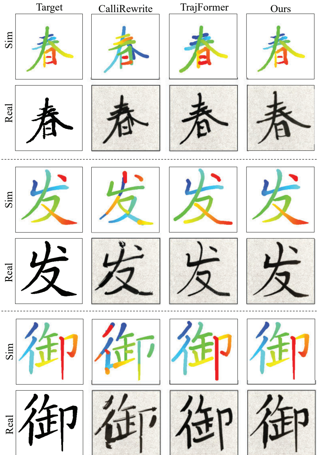
Figure 11. Comparisons on robotic demonstration. Each row of “Sim” showcases the trajectories of the target and the generated character, and “Real” represents the real character image and the robot rewriting results on different methods.
