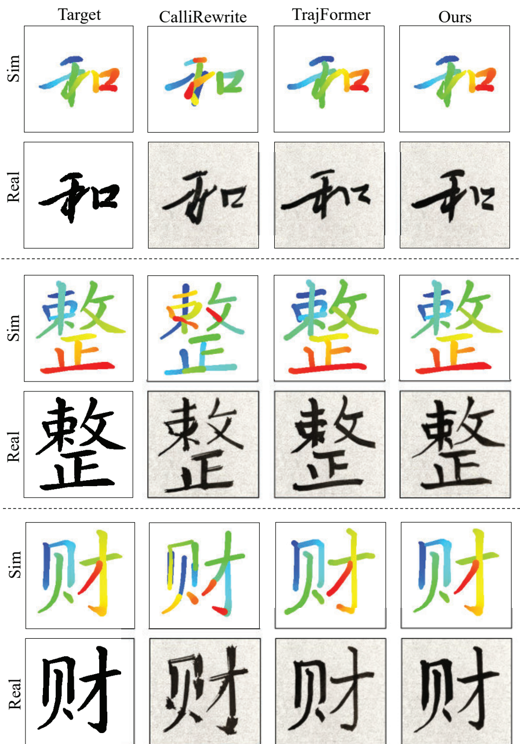
Figure 12. Comparisons on robotic demonstration. Each row of “Sim” showcases the trajectories of the target and the generated character, and “Real” represents the real character image and the robot rewriting results on different methods.
