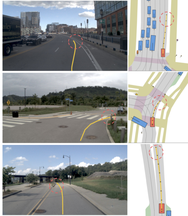
Figure 13. Failure cases of NORD. The predicted trajectory is shown in red and the violations marked in red circle.
