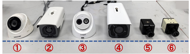
Figure B1. The six commercial-off-the-shelf cameras used for power signal injection.
