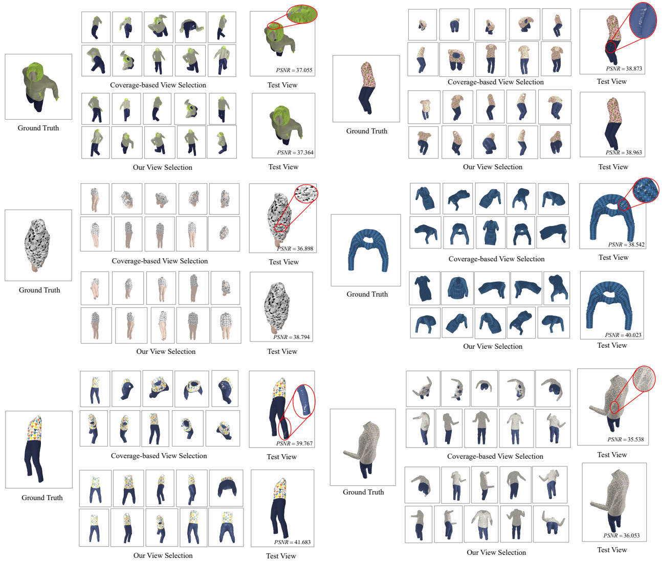
Figure 4. We compare the 10 views selected by the coverage-based strategy with those selected by our strategy. We then choose the worst viewpoint as the test view and compute its PSNR.
