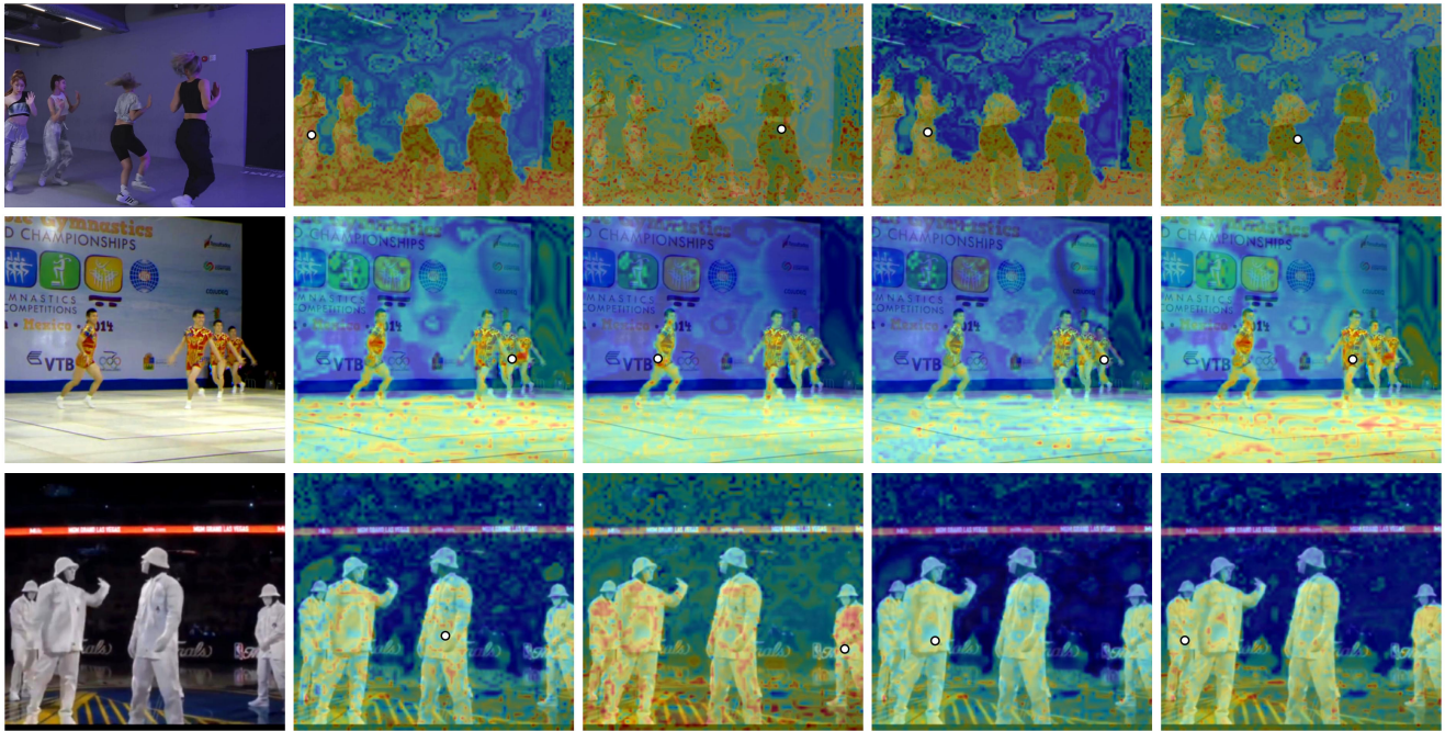
Figure 11. Visualizations of attention maps in SA. The first column denotes the input image, and the last four columns denote the attention maps of the target queries (denoted as white dots). Warmer colors indicate higher attention weights.
