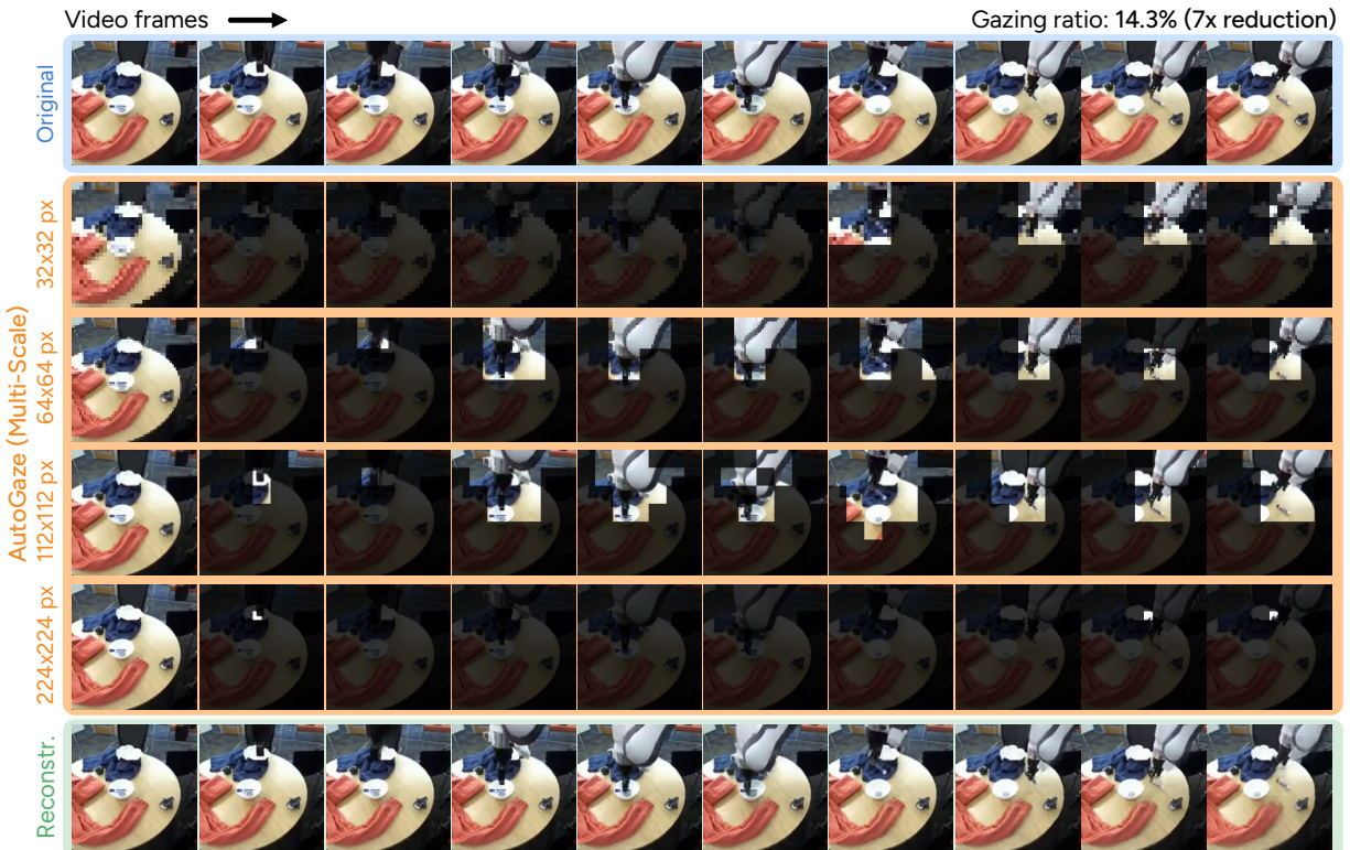
Figure 25. Robot arm video. AutoGaze uses different scales to gaze at the robot arm and marker.
