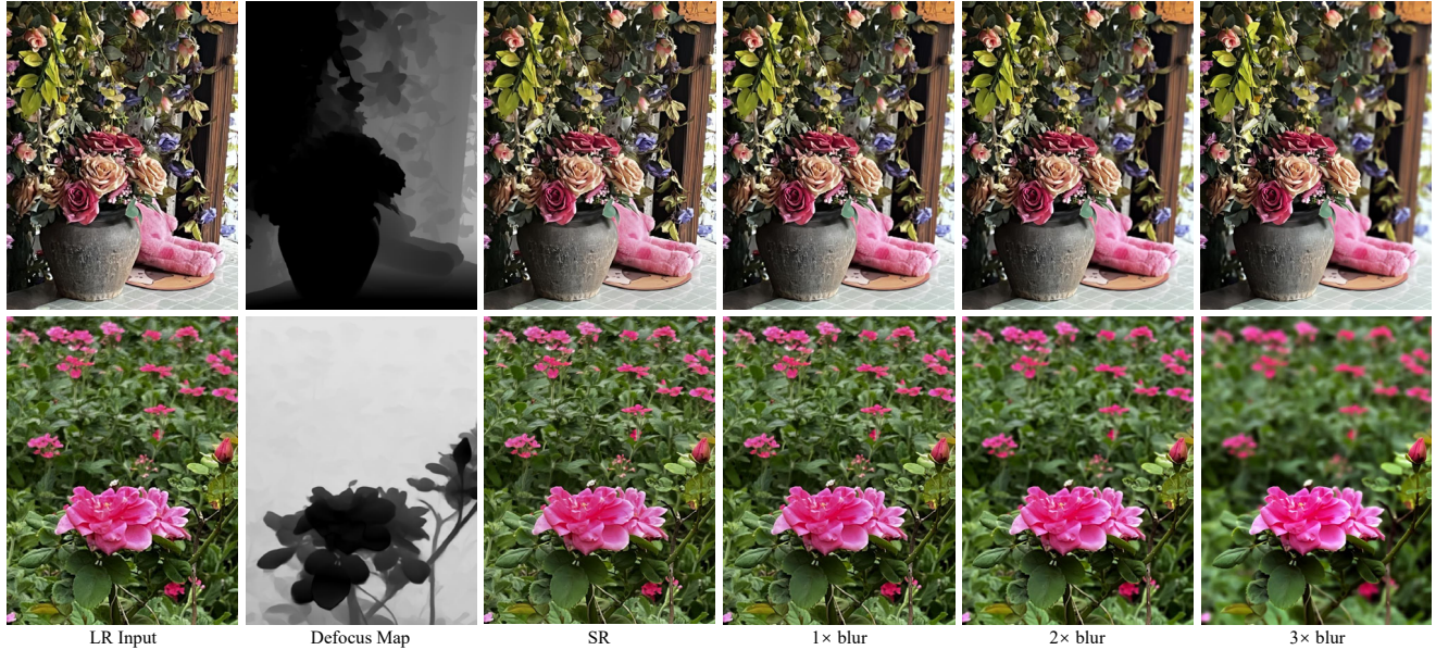
Figure 3. Given the defocus map and LR input, our method is able to gradually increase the aperture parameter from 1x blur to 3x blur ( Zoom-in for best view ).
