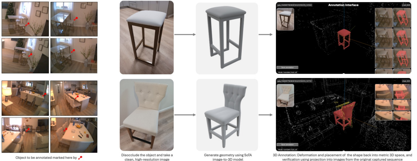
Figure 3. To obtain pseudo-ground truth geometry for an object in the sequence (left), we first place the object in isolation to avoid clutter and occlusion, and capture a high-quality, uncluttered image. We then apply segmentation and image-to-3D modeling to generate the object’s geometry (mid). This geometry is manually aligned and inserted back into the original casual sequence using a web annotation interface, verified by matching 2D projections to image silhouettes and by checking alignment with the sequence’s point cloud (right).
