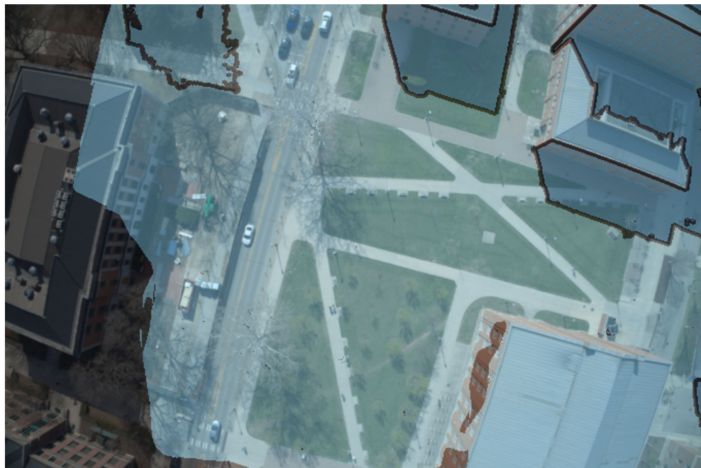
Figure D.1. Example of the binary confidence mask used during fine-tuning. The mask is constructed by combining geometry boundaries and shadow-projection boundaries. Blue regions indicate high-confidence supervision, while dimmer regions are excluded from training.
