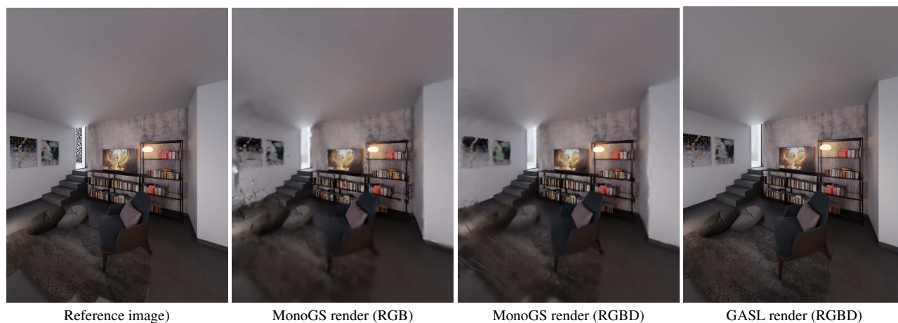
Figure S14. Groundtruth input and rendering results with other 3DGS-based SLAM methods in synthetic room sequence.
