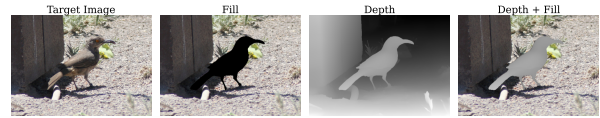
Figure A5. Mixed depth + fill control. The mixed control mode is a simple combination of the depth map and background fill image, where the mask is replaced with the pixels from the depth map.
