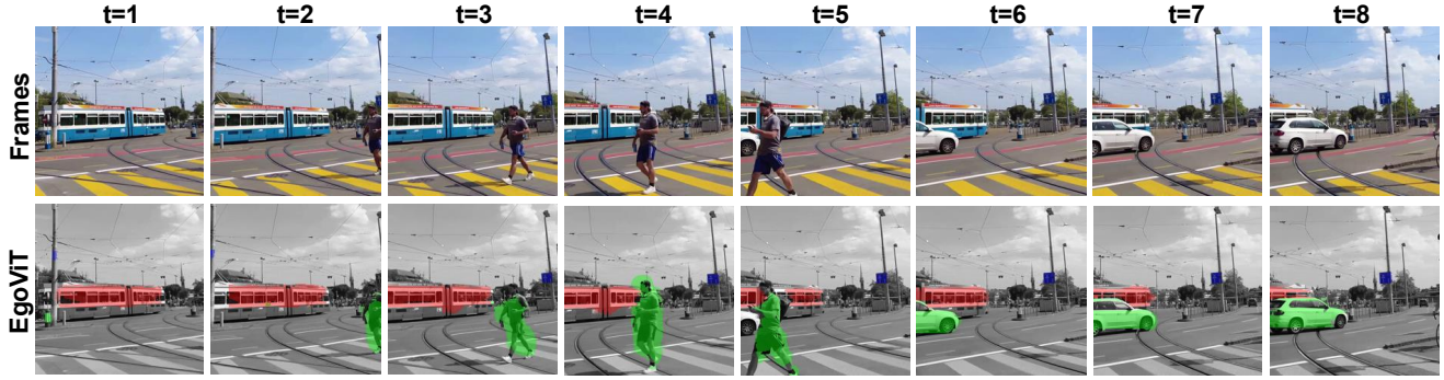
Figure 8. EgoViT maintains stable and distinct masks for the moving tram (red) and the pedestrian (green), effectively distinguishing them despite rapid camera panning and a cluttered background. When the pedestrian leaves the frame, the model seamlessly transitions to tracking the approaching car (also green). Additionally, EgoViT potentially exhibits partial capability in attending to small, distant objects, such as the signage (blue).
