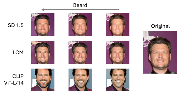
Figure 1. Editing in different latent spaces. The figure compares linear attribute editing across three latent spaces: two diffusion models and CLIP. The diffusion latents preserve the structure of the original image, so shifting along an attribute direction produces a modified version of the same image. In contrast, CLIP’s latent space is not invertible to the pixel domain, so reconstruction yields a newly synthesized image that matches the target attribute but does not reconstruct the input. This highlights the trade-off: CLIP offers strong semantic control but poor original image faithfulness.
