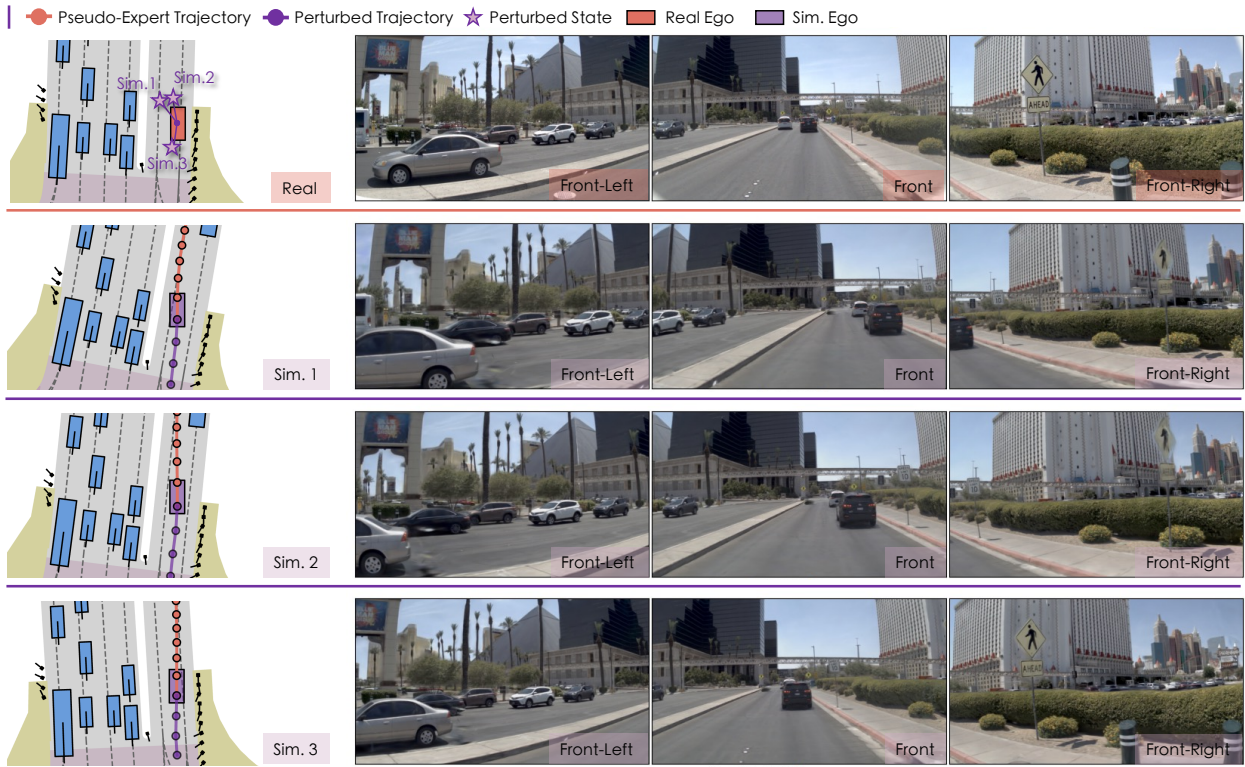
Figure 8. Qualitative results of planner-based expert with real and simulation data. (narrow local road)
