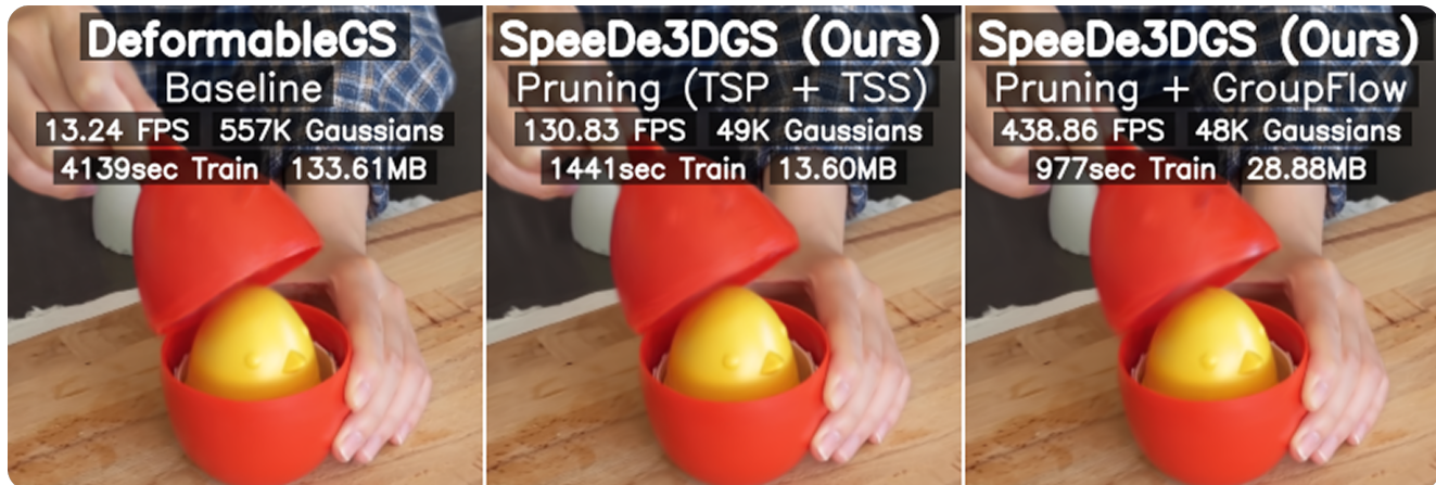
Figure 1. Our SpeeDe3DGS framework achieves 9.88\times faster rendering, 11.37\times fewer Gaussians, and 2.87\times shorter training on the HyperNeRF [37] chicken scene while preserving the image quality of DeformableGS [53] through Temporal Sensitivity Pruning (TSP) and Sampling (TSS). Applying our GroupFlow method on top of pruning accelerates rendering and training by 33.13\times and 4.24\times , respectively.
