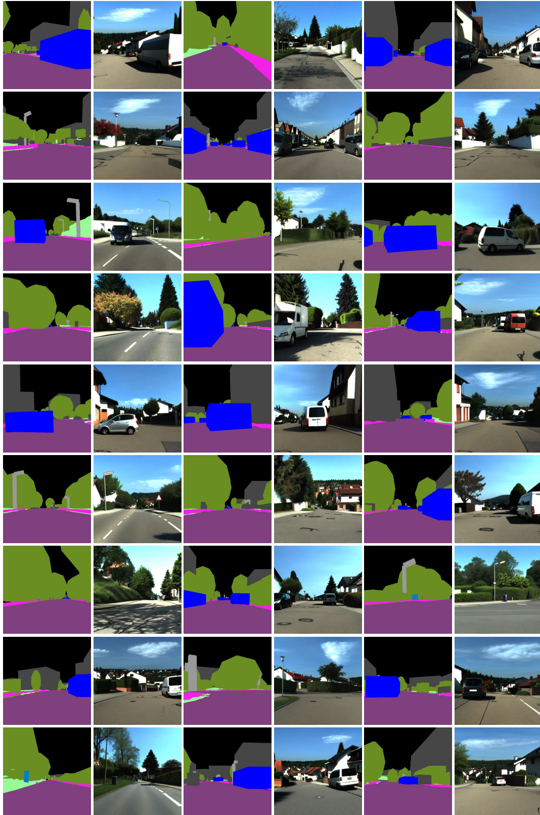
Figure 25. PrITI Photo-realistic Street View Synthesis Results. Each pair shows a 2D semantic rendering (left) and the corresponding photo-realistic image (right), generated with ControlNet [25]. Despite the coarse geometry of our primitives, the synthesized scenes exhibit diverse object appearances that go beyond cuboids or ellipsoids while remaining consistent with the input semantics.
