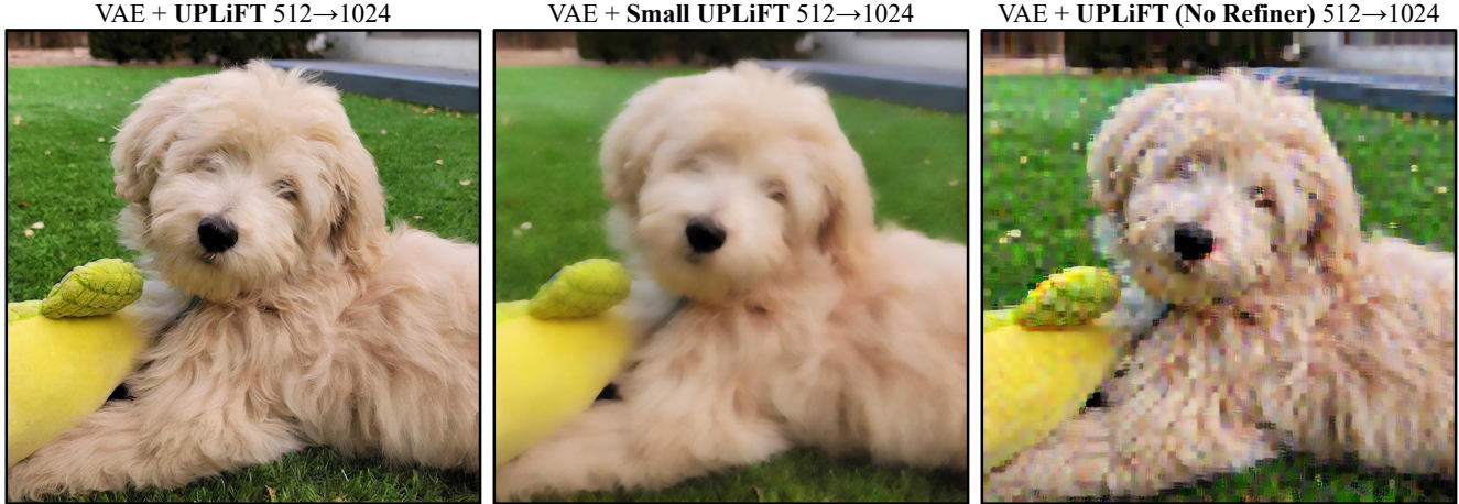
Figure 1. Visual ablation of design choices for VAE UPLiFT. (Left) UPLiFT achieves high quality 512→1024 upsampling with a larger parameter count model. (Middle) A smaller-scale UPLiFT has insufficient capacity to upsample all high-frequency information and produces blurry results. (Right) Ablation of the Refiner Block leads to blocky artifacts in upsampled images.
