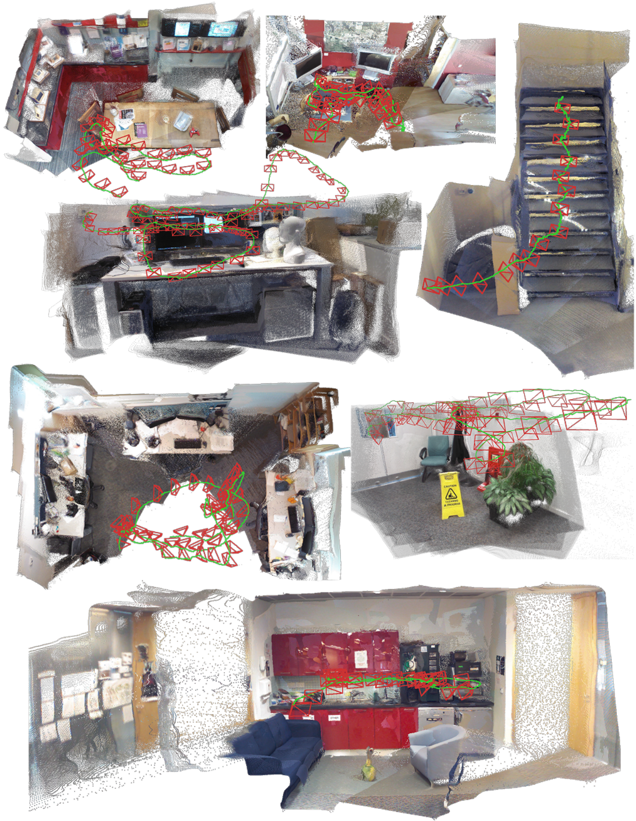
Figure 9. Qualitative showcase of VO on 7scenes [107]. We visualize keyframe poses as red cameras and non-keyframe poses as green dots.
