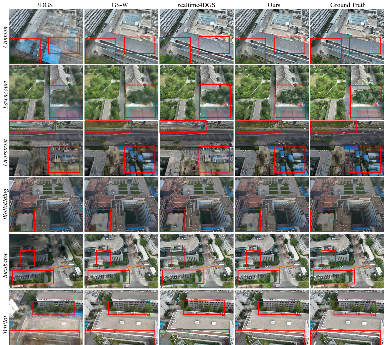
Figure 1. Qualitative comparison on real scenes of ChronoScene. We compare ChronoGS with representative baselines. Each row shows novel-view renderings of different methods, along with ground truth. Static models trained on mixed multi-period data produce ghosting and appearance blending due to inconsistent geometry, while dynamic methods that assume continuous motion fail under the large temporal gaps, causing incorrect geometry interpolation. ChronoGS faithfully reconstructs period-specific geometry and appearance, preserving sharp, temporally consistent details across long-term changes.
