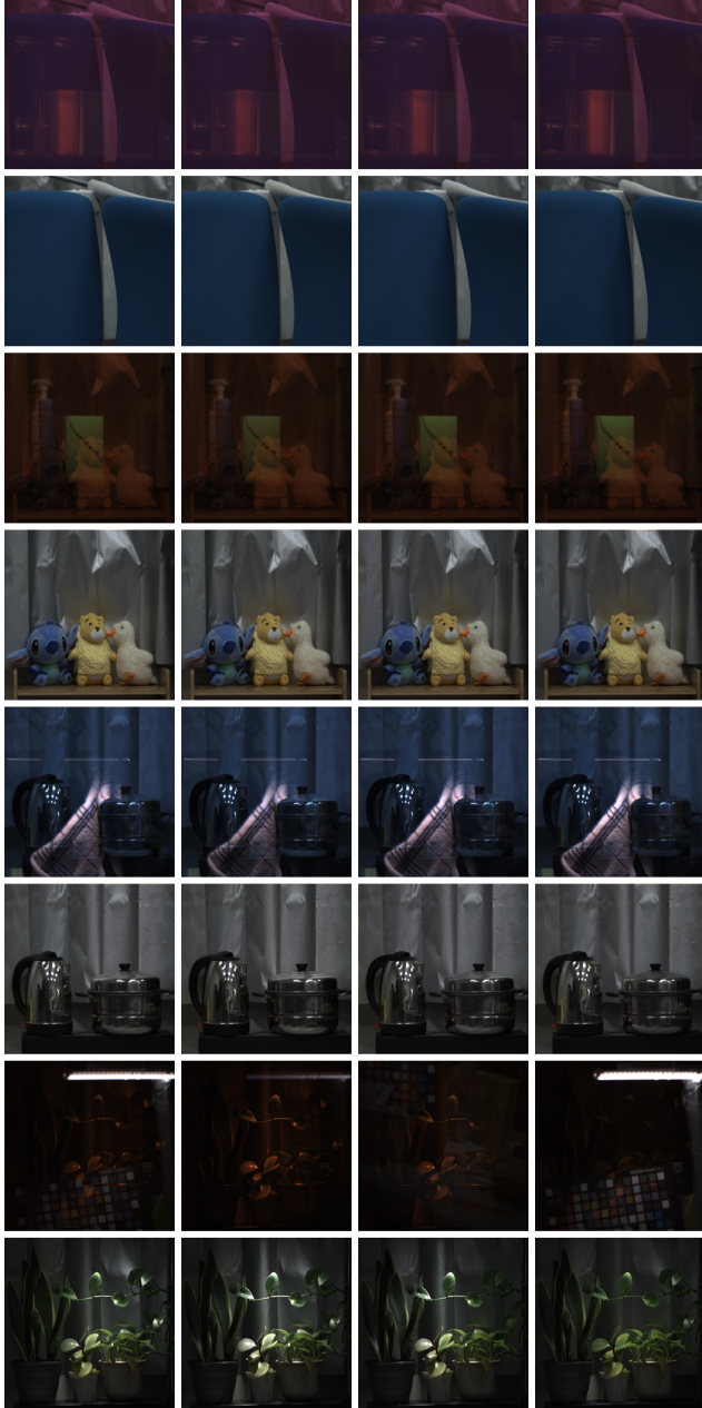
Figure 4. Visualization of representative scenes from our GlassPol dataset. Each column corresponds to one of the four polarization orientations ( 0^\circ , 45^\circ , 90^\circ , 135^\circ ) captured simultaneously by the micro-polarizer array in a single shot. From top to bottom: chair , dolls , kettle , and plants . These scenes cover diverse materials such as diffuse surfaces, glossy regions, and mixed reflection types, providing broad coverage of real-world polarization behaviors.
