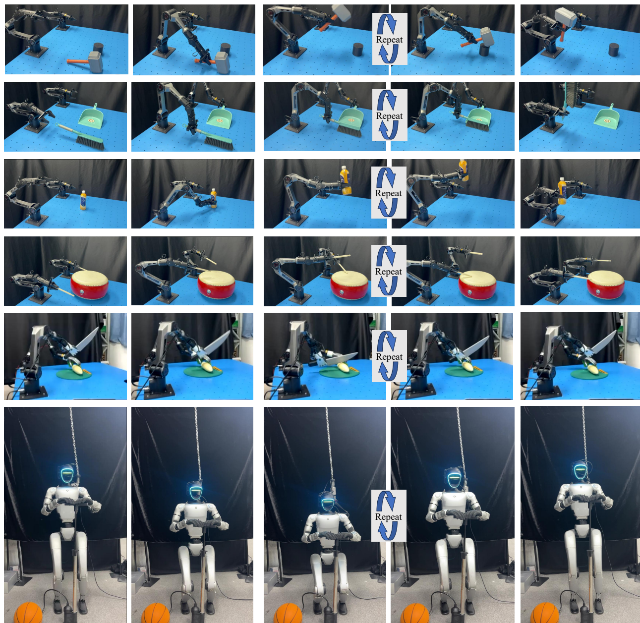
Figure 5. Visualization of autonomous inference of our framework in real world. To reduce space usage, we omit the loop frames and display only a single loop action.
